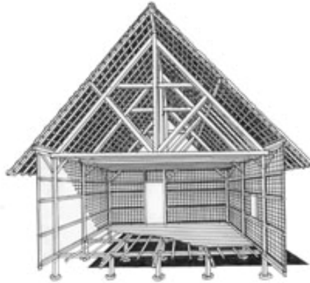
Figure 3: Perspective section of box frame
